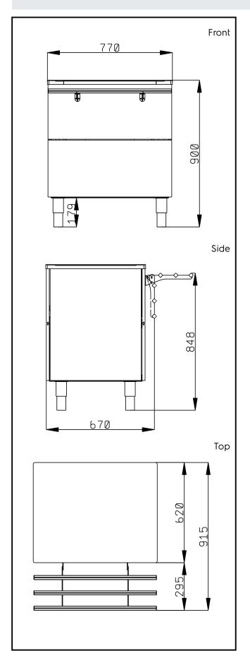
Flexy Compact Ambient Unit on cupboard (2 GN) with one stainless steel tray slider
